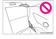
Always make sure that the seatbelt is not caught in the seatback or twisted in one of the hooks that secure the seatback. Failure to do so may cause the seatbelt to not be fastened correctly or to become ineffective in a collision, resulting in serious injury. 1-3. Adjustable components (seats, mirrors, steering wheel) Head restraints
