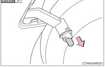
Pull out the lamp and turn the lens counterclockwise.
