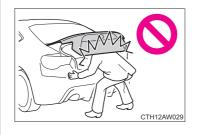
• The trunk lid may fall if it is not opened fully. It is more difficult to open or close the trunk lid on an incline than on a level surface, so beware of the trunk lid unexpectedly opening or closing by itself. Make sure that the trunk lid is fully open and secure before using the trunk. 1 Before driving
